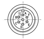
Mating connector according to DIN EN 175201-804 separate order under the Material no. **R900223890** (metal version)
