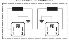
Mating connector CECC 75 301-803-A002FA-H3D08-G according to DIN EN 175301-803 and ISO 4400 Solenoid a, color gray separate order under the Material no. R901017010 Solenoid **b**, color black separate order under the Material no. R901017011
