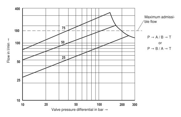
Observe the maximum admissible flow of 180 l/min!
