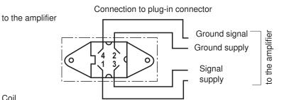
Mating connector 4-pole Pg7-G4W1F separate order under the Material no. R900023126 Connection cable:
