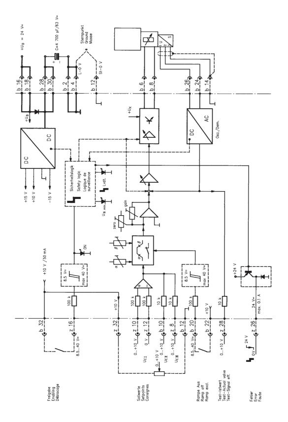
Versions of trigger electronics: - With ramps, see page 7 and RE 30052
