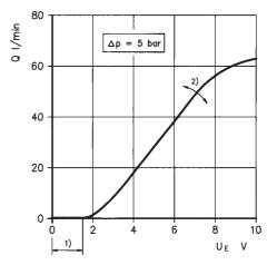
Valve amplifier <sup>1)</sup> Zero adjustment <sup>2)</sup> Sensitivity adjustment
