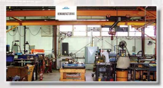
Product that has met core criteria for remanufacturing is received at a section of our Canfield, Ohio facility devoted to the REMAN process where it is torn down and parts are inspected to factory usability specifications.
